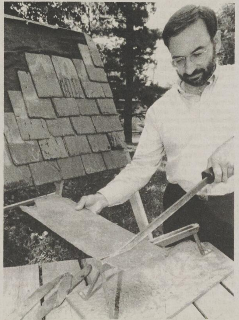
Pierre Bail demonstrates how slate is cut to make tiles with one of the tools on display at the slate interpretation centre.
