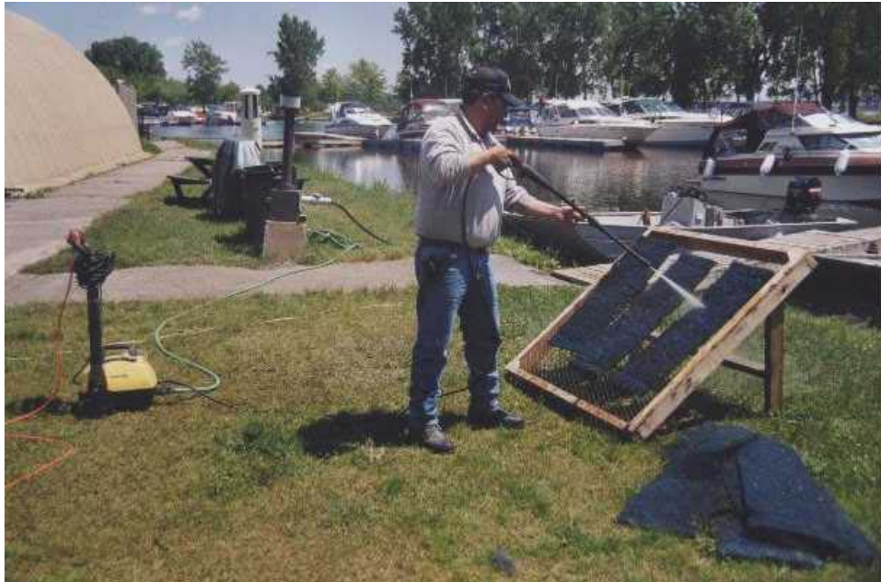
Photo 4. Parpen cleaning technique involving the use of a support and a high-pressure sprayer, upstream portion of the Lachine Rapids, spring of 2002.
