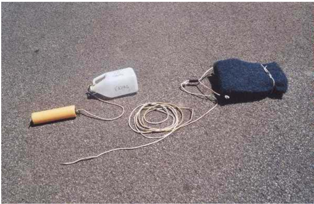
Photo 2. Assembled sampling gear; the parpen is covered with the piece of air filter which is held in place by the elastic band.
