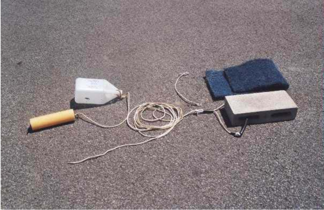
Photo 1. Elements making up the sampling gear used for the systematic search for lake sturgeon eggs in the upstream portion of the Lachine Rapids, spring of 2002: cement parpen, piece of air filter, elastic band with hooks, rope and floats.
