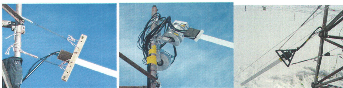
Figure 18 - Suspension of the snow cable sensor for winter 2001/02 (left), winter 2002/03 (middle) and winter 2003/2004 (right).
